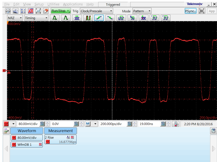
Figure 7: 10 Gbps PRBS pattern as applied to the HL9404 RF In port
