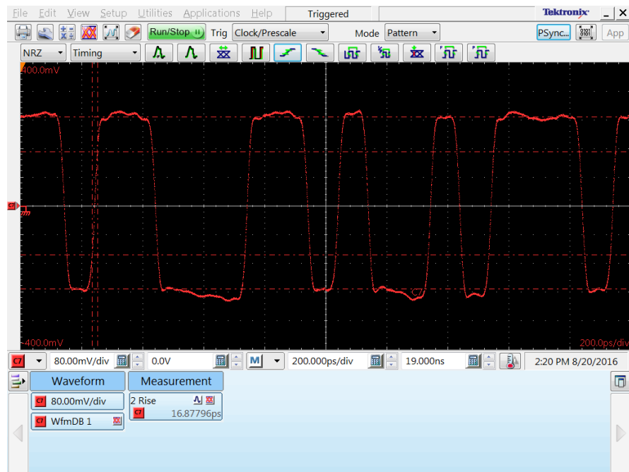
Figure 8: 10 Gbps PRBS pattern as applied to the HL9407 RF In port
